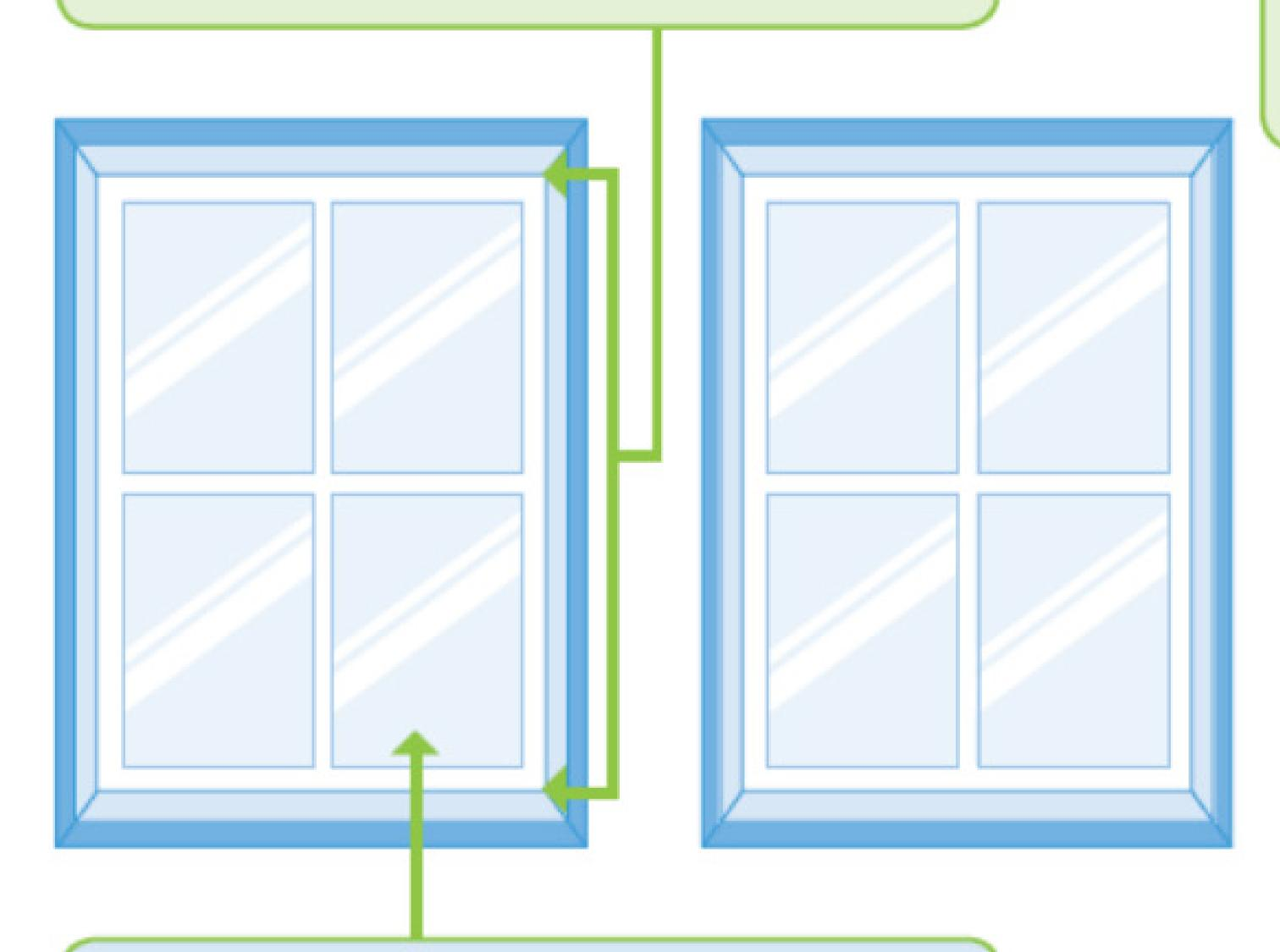
Second, the path that sound takes through a window is the glass itself. Sound travels through a medium (air, wood, glass, aluminum, etc.) as vibrations. Generally, the heavier or stiffer an object is, the more resistant it is to vibration. The type of glass that is used can also have an effect on noise reduction. Laminated glass can be effective at reducing noise. Windows designed for airport sound insulation programs are usually made of vinyl or aluminum.
